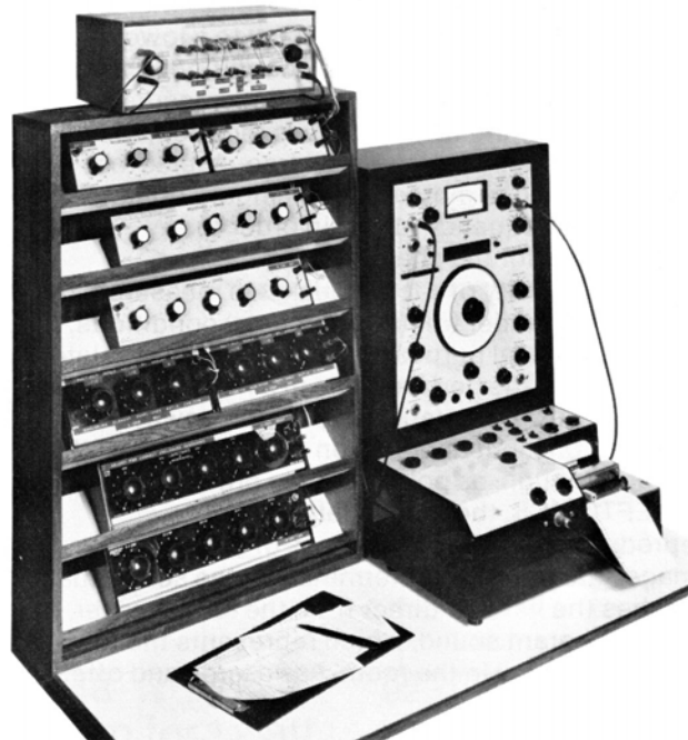
Fig. 3. Electrical simulator for demonstrating effect of varying loudspeaker parameters.
